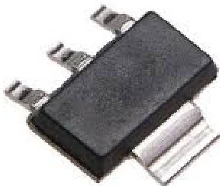
BCP53 Transistor bipolaire (BJT) PNP, -80 V, 1.5 W, -1.2 A, 25 hFE SOT-223
